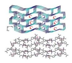
A (10,3)-d metal-organic framework,  $[Mn_2(pdtd)_2(H_2O)_4]_n$ - $5nH_2O$  (1), containing the asymmetrical 3-(2-pyridyl)-5,6-diphenyl-1,2,4-triazine-P,P'-disulfonate ligand (pdtd) was constructed. XRD analysis revealed that 1 is an acentric structure possessing exposed uncoordinated nitrogen atoms within helical cavities. 1 exhibits multifunctionality: nonlinear optical activity,  $CO_2$  sorption, and magnetic coupling.
