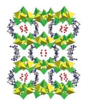
Three new beryllium phosphite solids have been prepared in the presence of different amine molecules as the structure-directing agents. These compounds represent the first examples of open-framework beryllium phosphites with layered structures.
